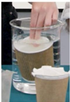
Put your cup in a bowl or beaker of water. Fill the cup with water so it sinks.
