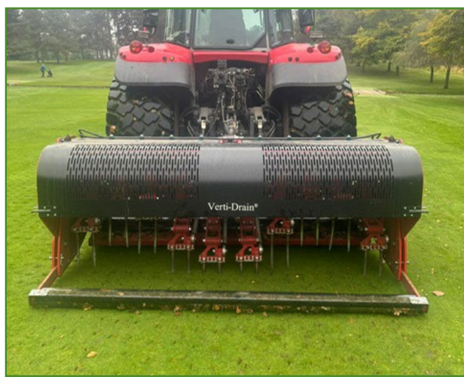
Figure 2. An aerating machine puts holes in the ground to let water drain away. © Birmingham County FA
