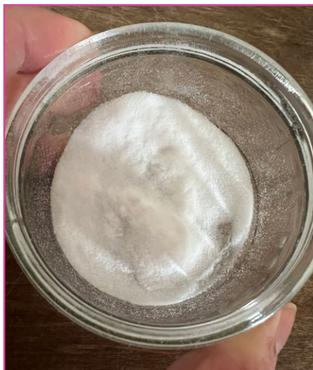
Figure 3. Hollow glass microspheres © Dr R Ellis, PSTT
