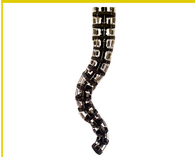
Figure 1. An elephant trunk robotic arm which is operated by a system of guide wires and springs.
