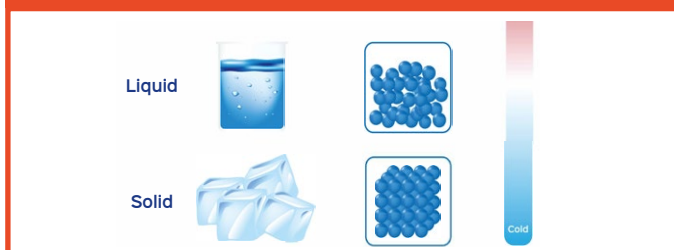
Figure 2. Particles in a solid are arranged uniformly and tightly packed. In a liquid, the particles are still closely but less uniformly arranged and move around each other (flow).
