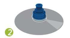
Push the bottle top down onto the CD so that it sticks to the CD with no gaps for the air to escape.
