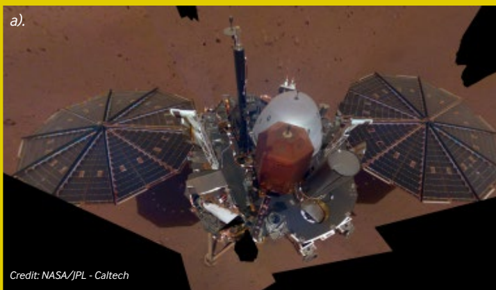
Figure 1. a). NASA InSight's first 'selfie' and b). InSight's scoop pushes on top of the 'mole', InSight's Heat Flow and Physical Properties Package, a self-hammering heat probe that measures the heat flowing from the planet.
