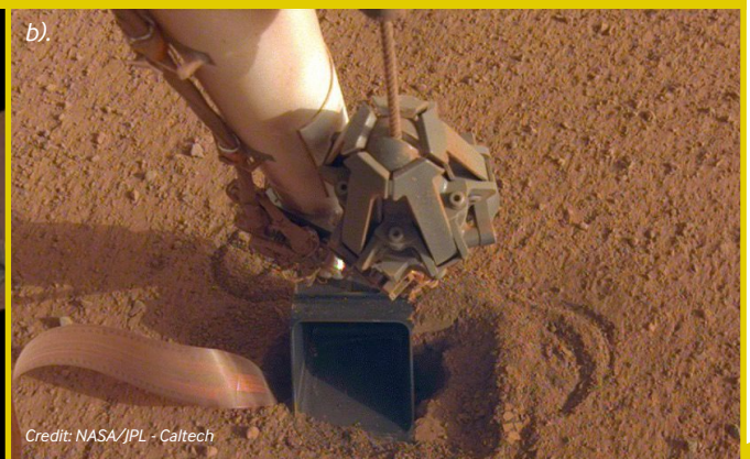
Figure 1. a). NASA InSight's first 'selfie' and b). InSight's scoop pushes on top of the 'mole', InSight's Heat Flow and Physical Properties Package, a self-hammering heat probe that measures the heat flowing from the planet.
