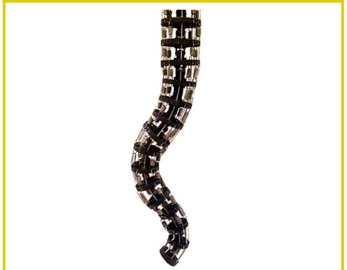
Figure 1. An elephant trunk robotic arm which is operated by a system of guide wires and springs.
