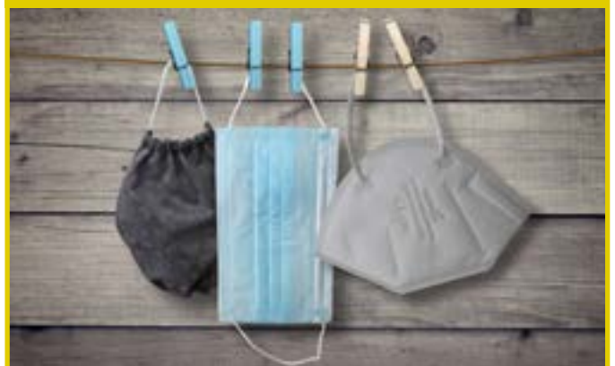
Figure 3. Different types of face masks (from left to right): a homemade woven cotton mask which could have one or more layers, a surgical mask has three-layers of nonwoven plastic (polypropylene), a 'filtering facepiece' (FFP2) has four-layer protection. The cotton facemask can be washed and reused but the others are non-reusable.
