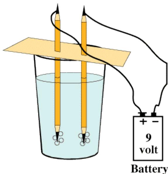
Experimental set-up (with pencils instead of graphite rods)
